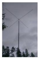
weather. The Spiderbeam is a wire beam and was totaly filled with ice and snow and looks like totaly destroyed. Eventually the antenna was still perfectly resonant. He works perfect on whole WARC bands.
